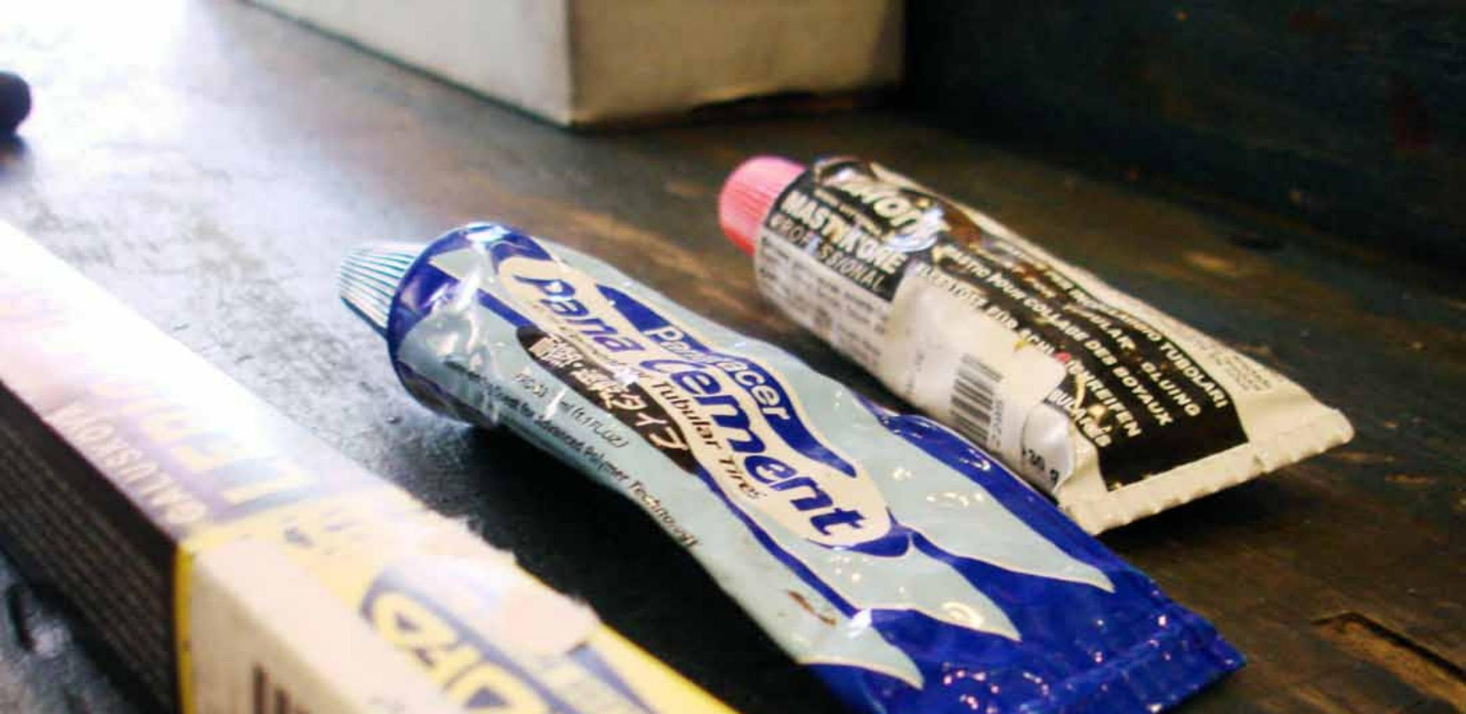
There are many types of glues used in putting tubulars together. In our situation we use Panaracer Pana Cement. We do not recommend using tape on wheels to start off. For spares it can be used but also, not recommended by us, we believe in properly preparing a spare tire the same way we prepare the tire here.
