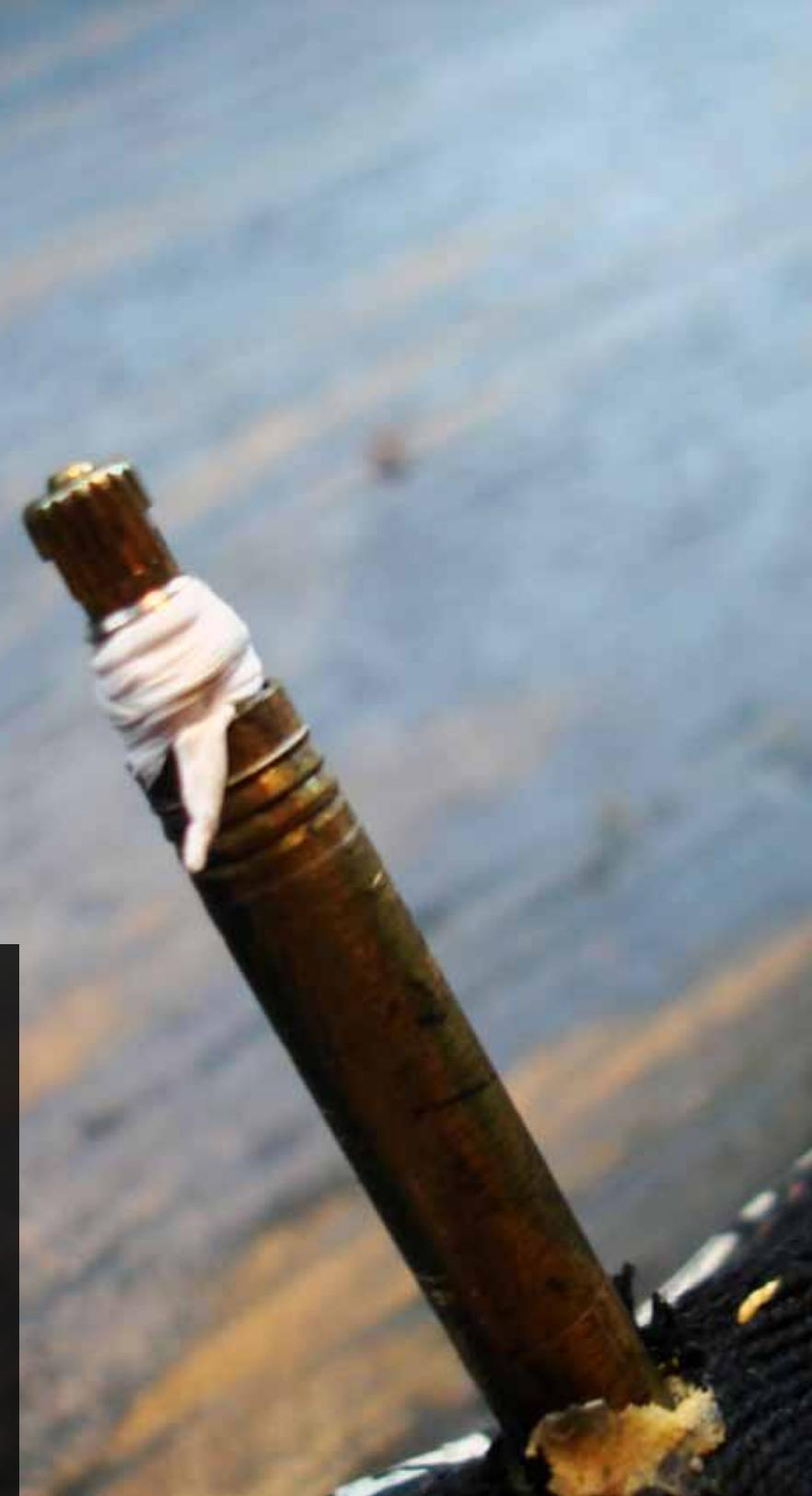
Having the valve tight and locked out will help prevent to take the valve extender off to service the valve itself because sometimes if not properly prepared can loosen later in life. Then, take approximately 3 centimetres worth of plumbers tape and wrap it around the threads tightly for a proper seal on the extender.
