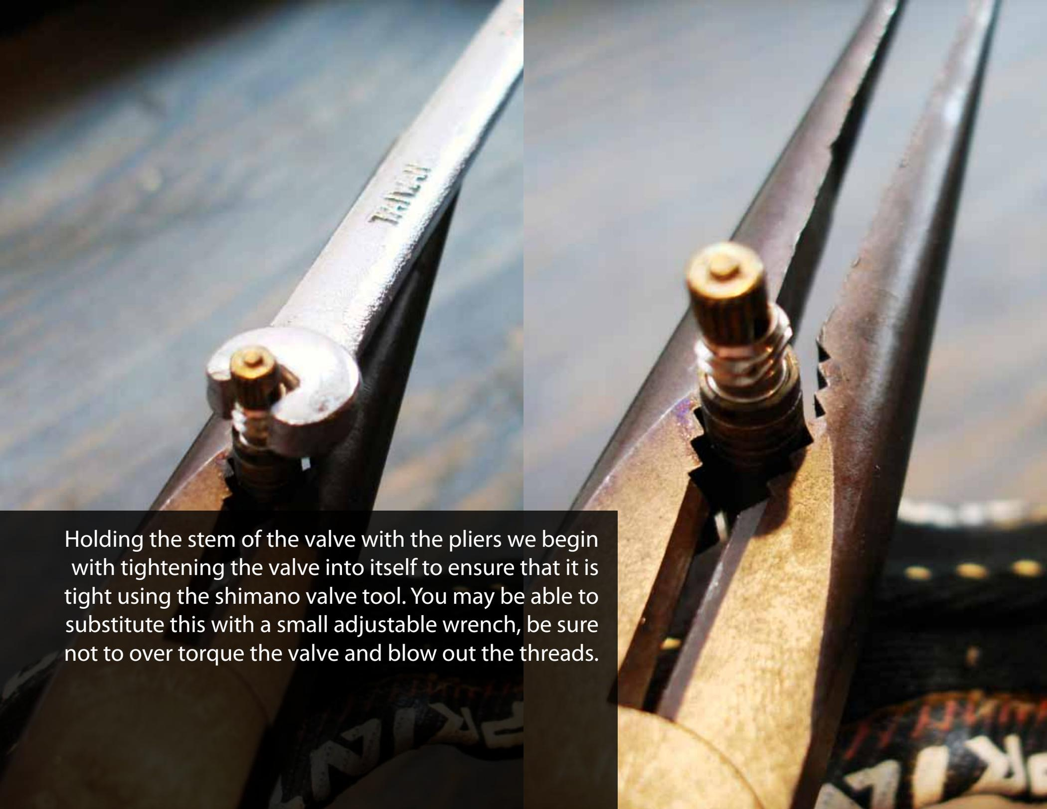
Holding the stem of the valve with the pliers we begin with tightening the valve into itself to ensure that it is tight using the shimano valve tool. You may be able to substitute this with a small adjustable wrench, be sure not to over torque the valve and blow out the threads.
