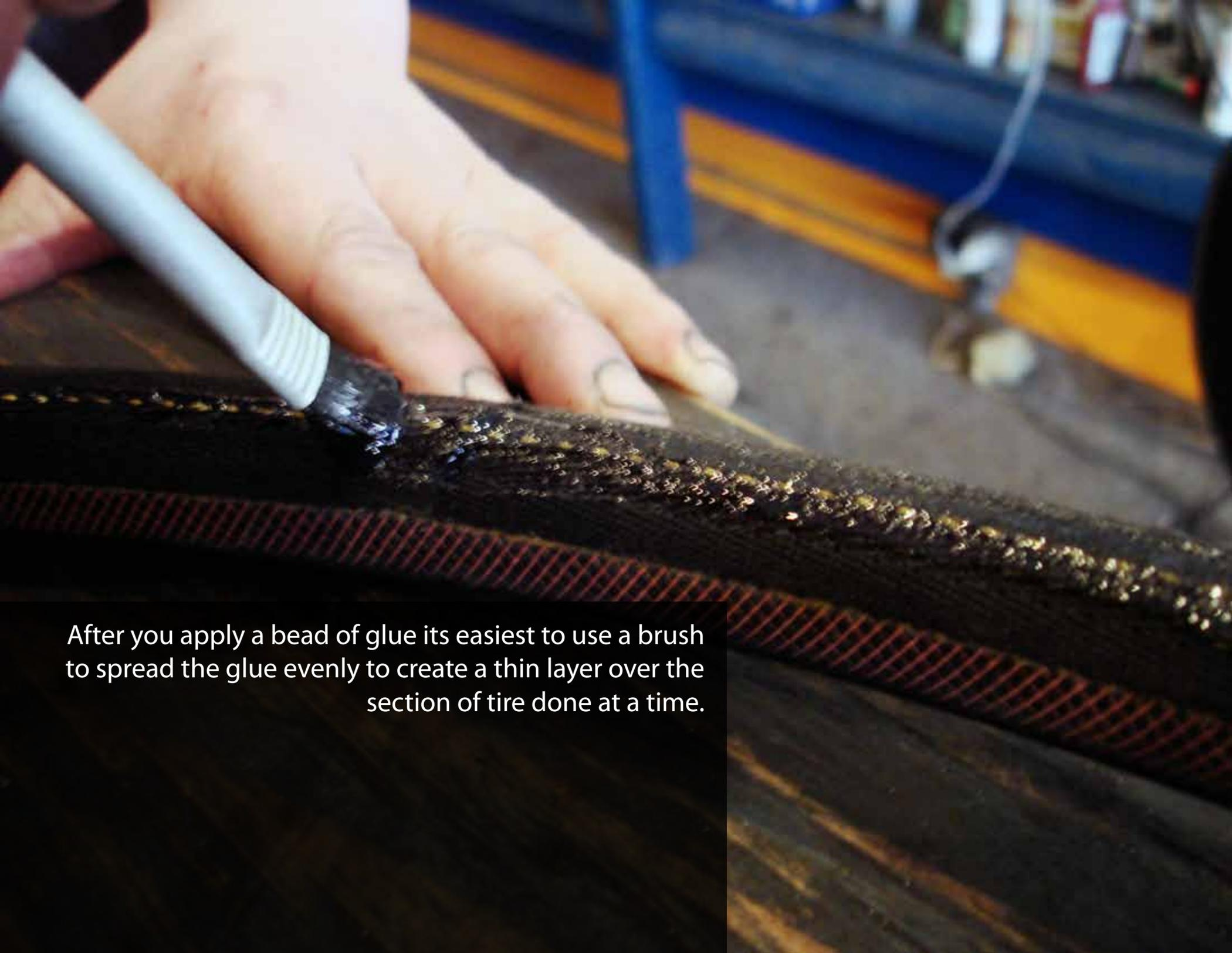
After you apply a bead of glue its easiest to use a brush to spread the glue evenly to create a thin layer over the section of tire done at a time.
