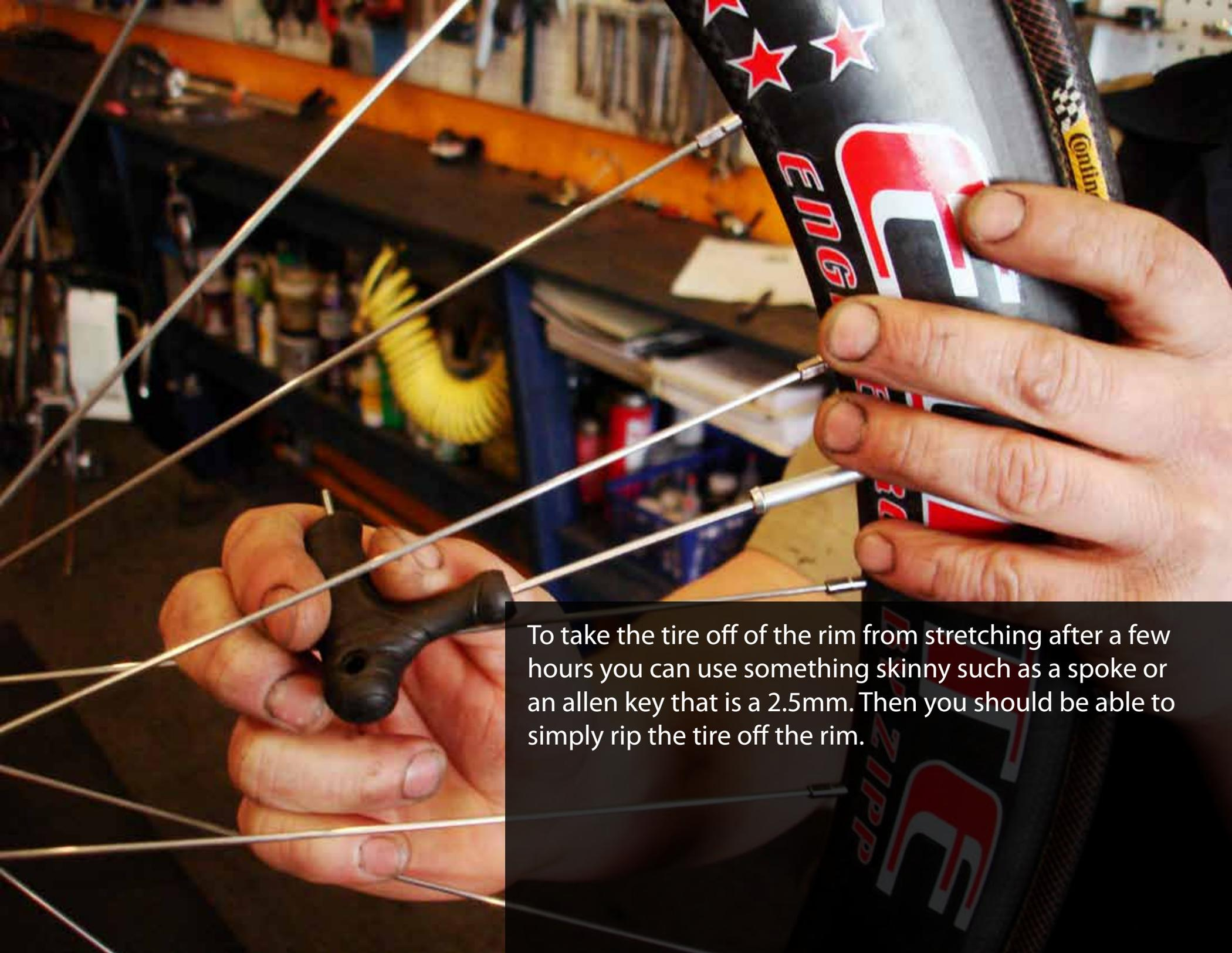
To take the tire off of the rim from stretching after a few hours you can use something skinny such as a spoke or an allen key that is a 2.5mm. Then you should be able to simply rip the tire off the rim.
