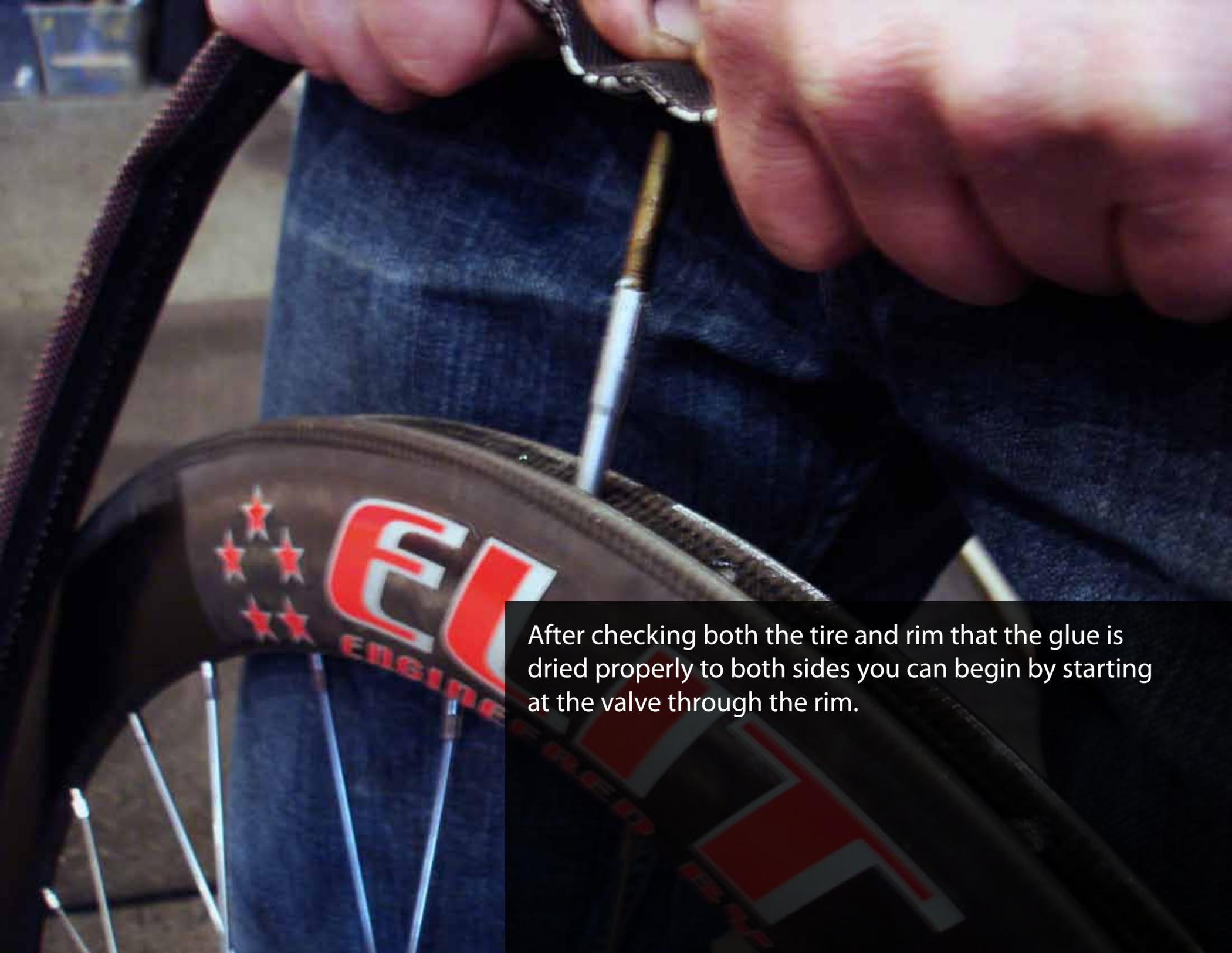
After checking both the tire and rim that the glue is dried properly to both sides you can begin by starting at the valve through the rim.
