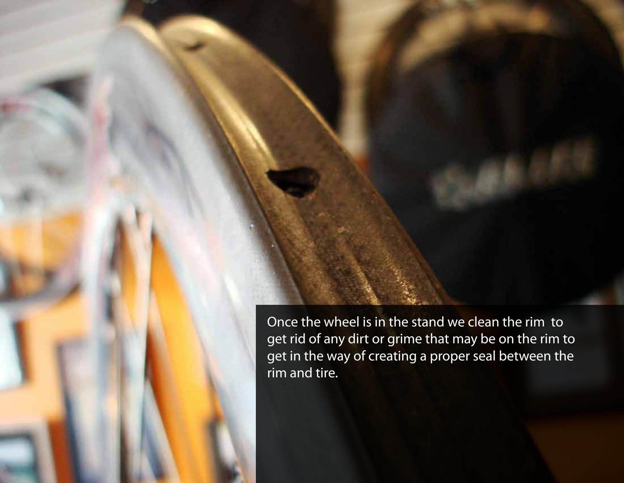
Once the wheel is in the stand we clean the rim to get rid of any dirt or grime that may be on the rim to get in the way of creating a proper seal between the rim and tire.
