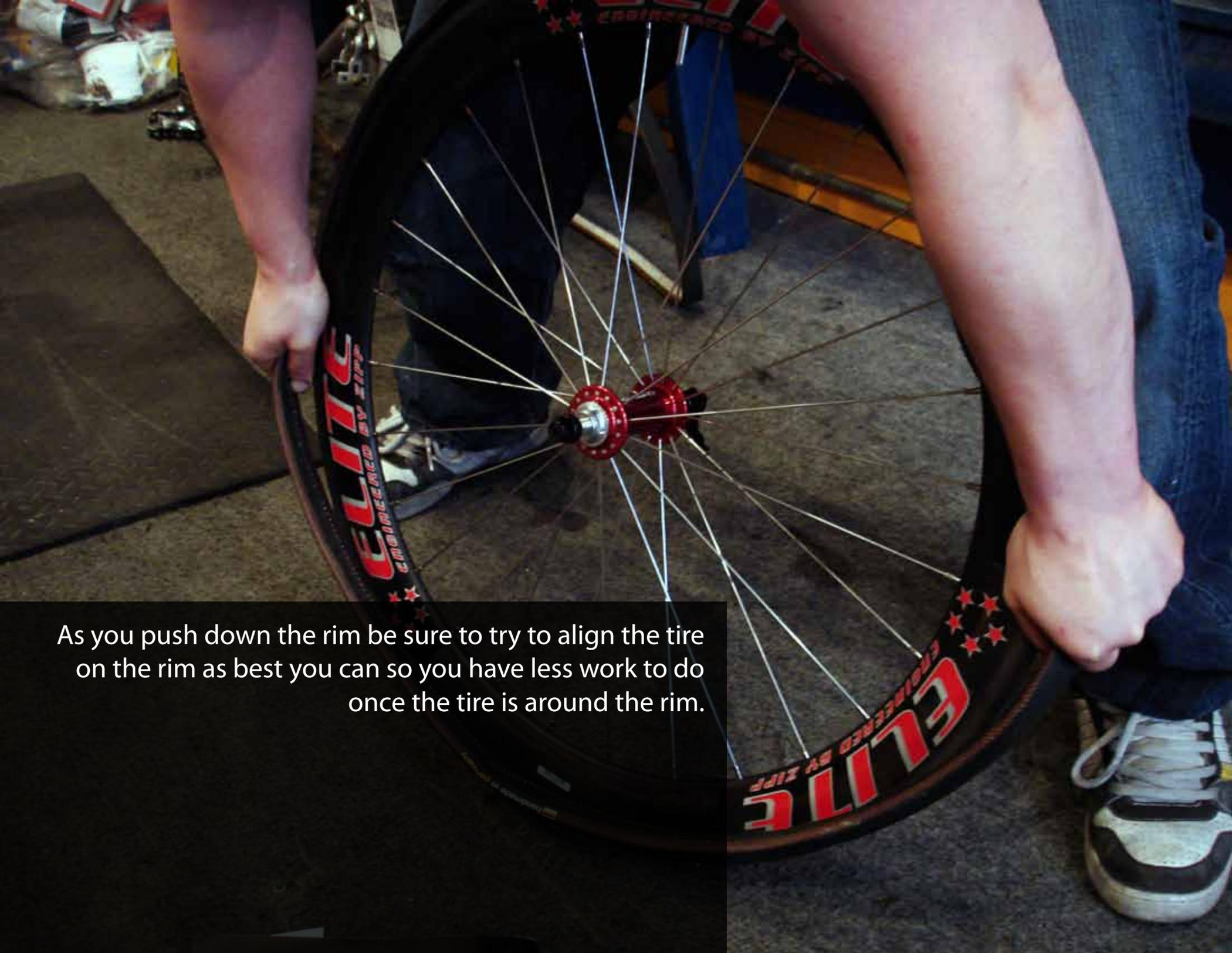
As you push down the rim be sure to try to align the tire on the rim as best you can so you have less work to do once the tire is around the rim.
