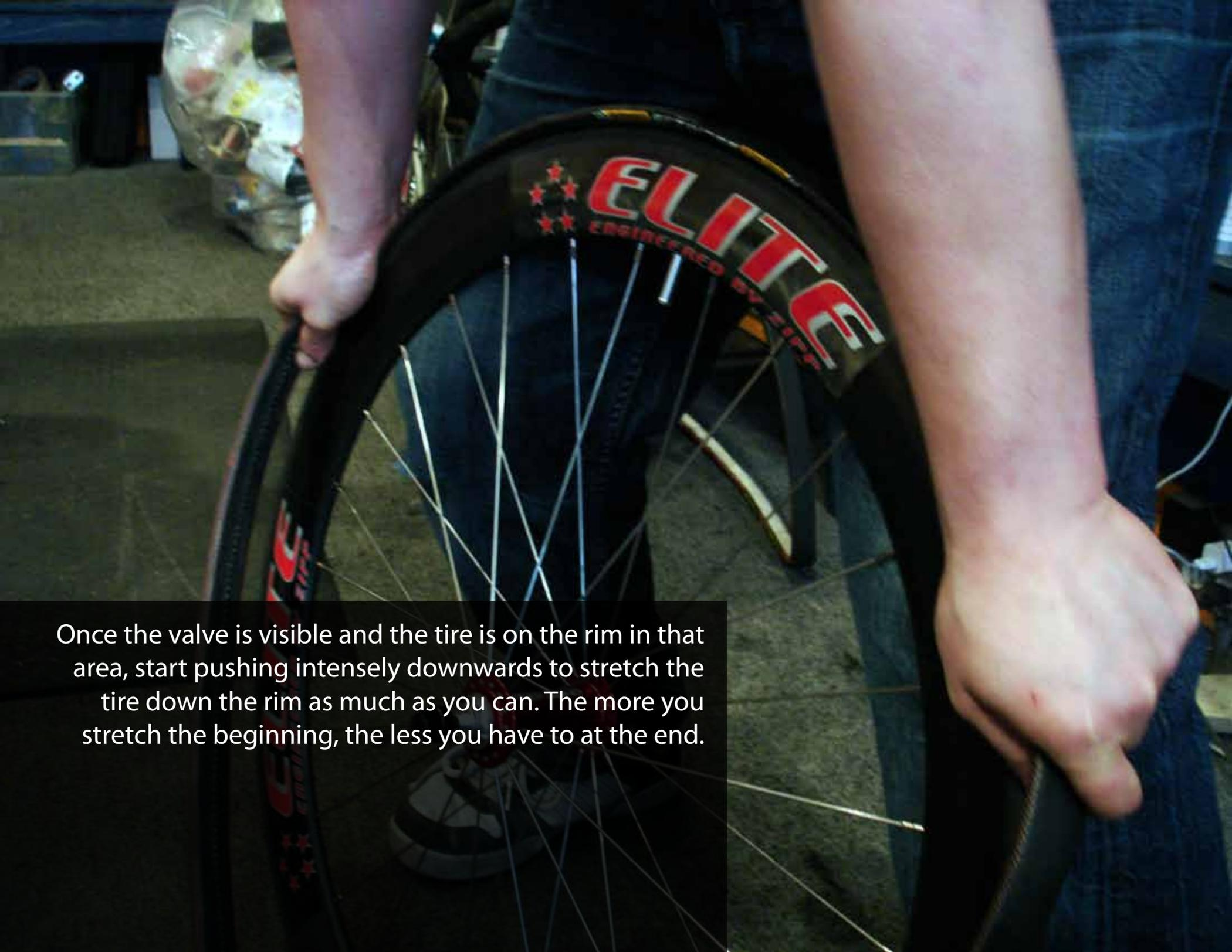
Once the valve is visible and the tire is on the rim in that area, start pushing intensely downwards to stretch the tire down the rim as much as you can. The more you stretch the beginning, the less you have to at the end.
