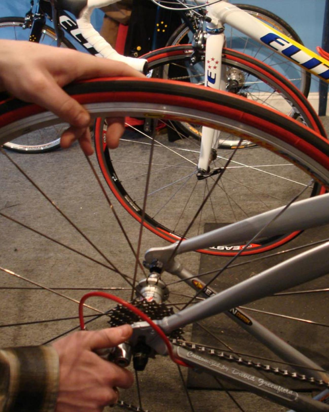
Here you see the derailleur out of the way while the wheel is coming out of the drop outs as to not scratch or interfere with one another.
