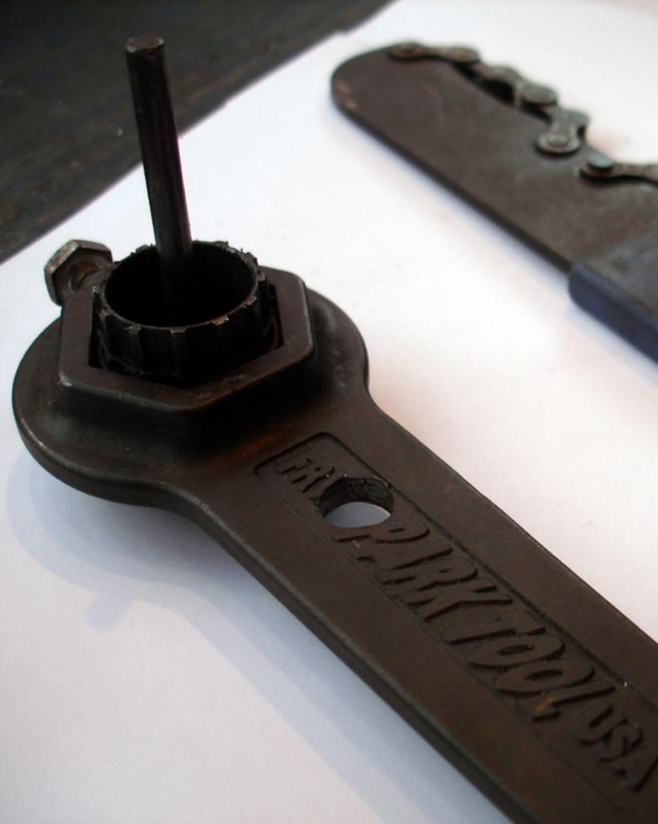
Now apply the Lockring Tool by inserting the end of the tool where the skewer goes and slide it into the cassette until feel the teeth slide into the lockring itself. The lockring tool should be on the opposing side of the chainwhip, which should be in your right hand.
