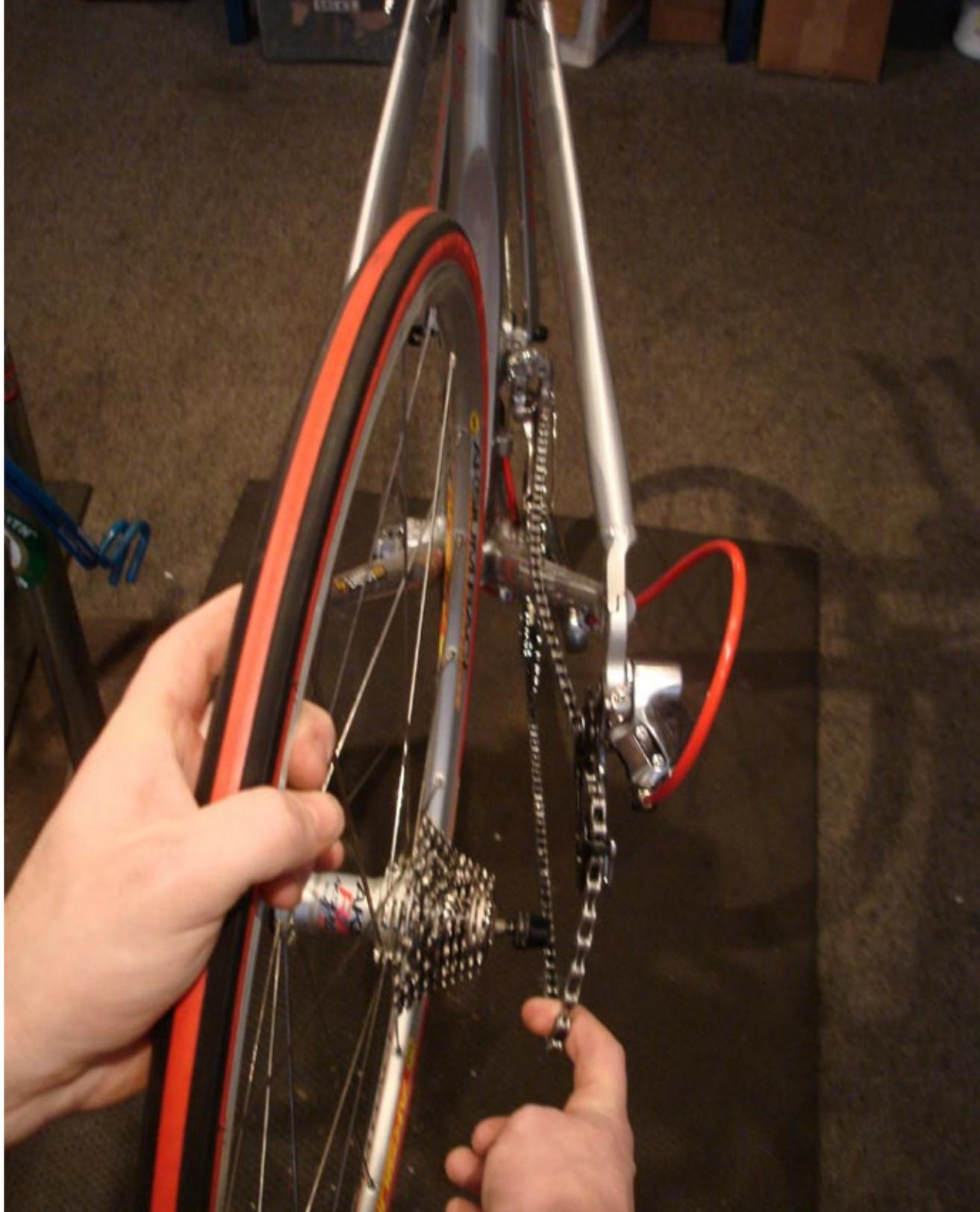
After the wheel is taken out the next step is to remove the skewer by unscrewing until the cap comes off with a spring underneath.
