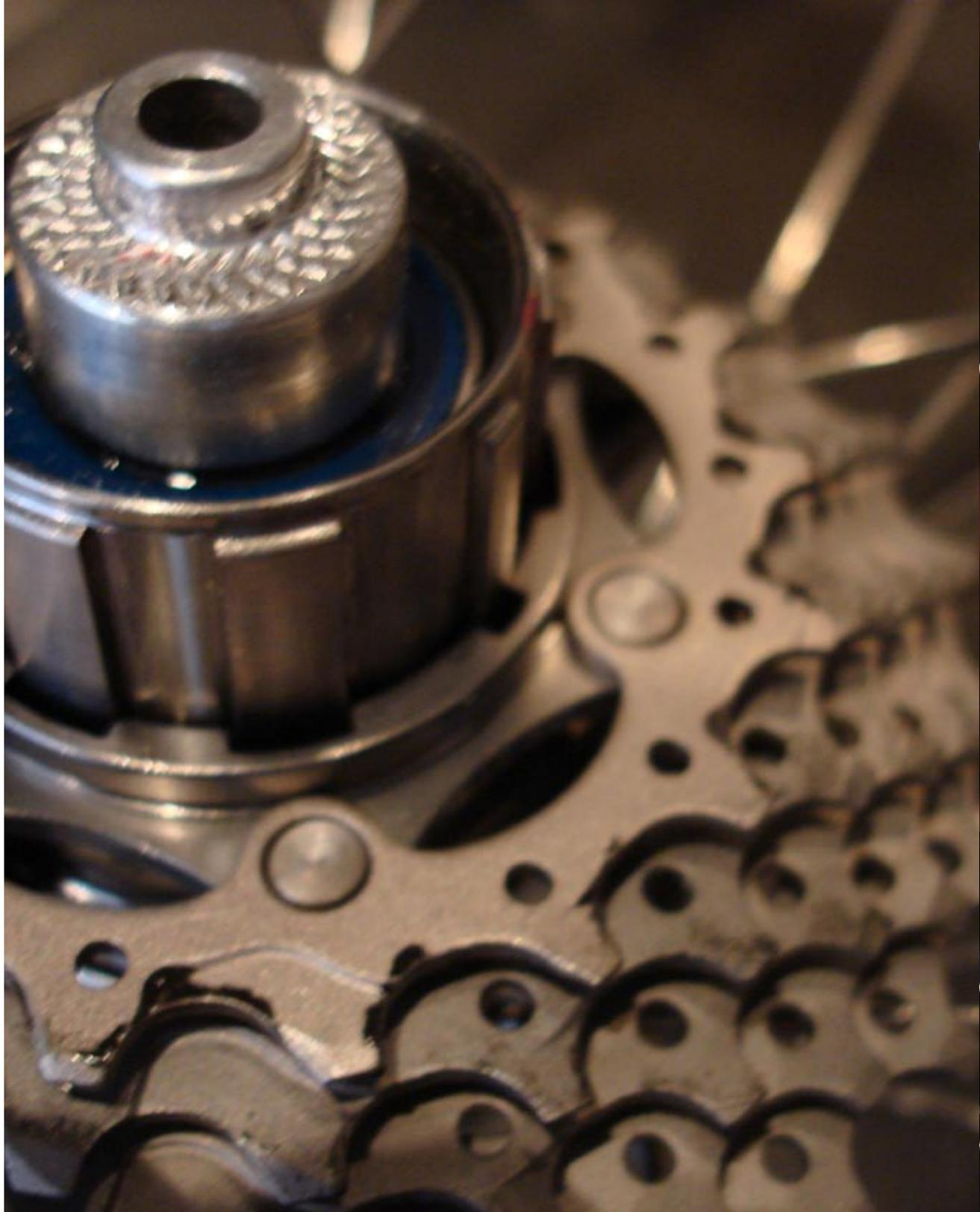
On a Dura-ace ten speed cassette the next few have separate spacers from cogs. It starts with the next cog, then a spacer that is labeled "10S" for ten speed cassettes.
