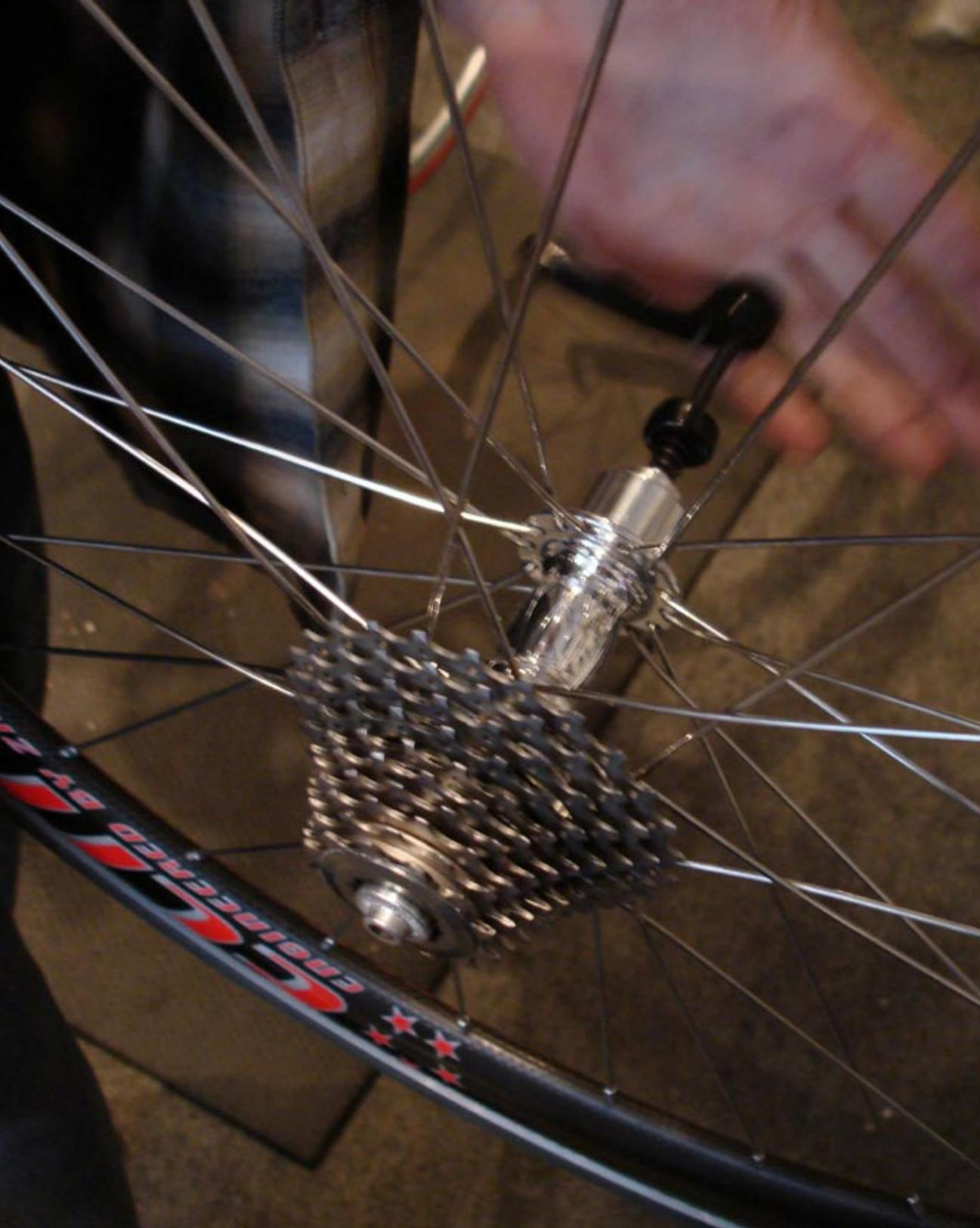
Take your skewer from the training wheel, unless you have a race skewer and slide back through the wheel with the handle on the non-drive side of the wheel. Make sure there is grease on the skewer and its threads to prevent it from freezing from sweat and elements affecting the skewer.
