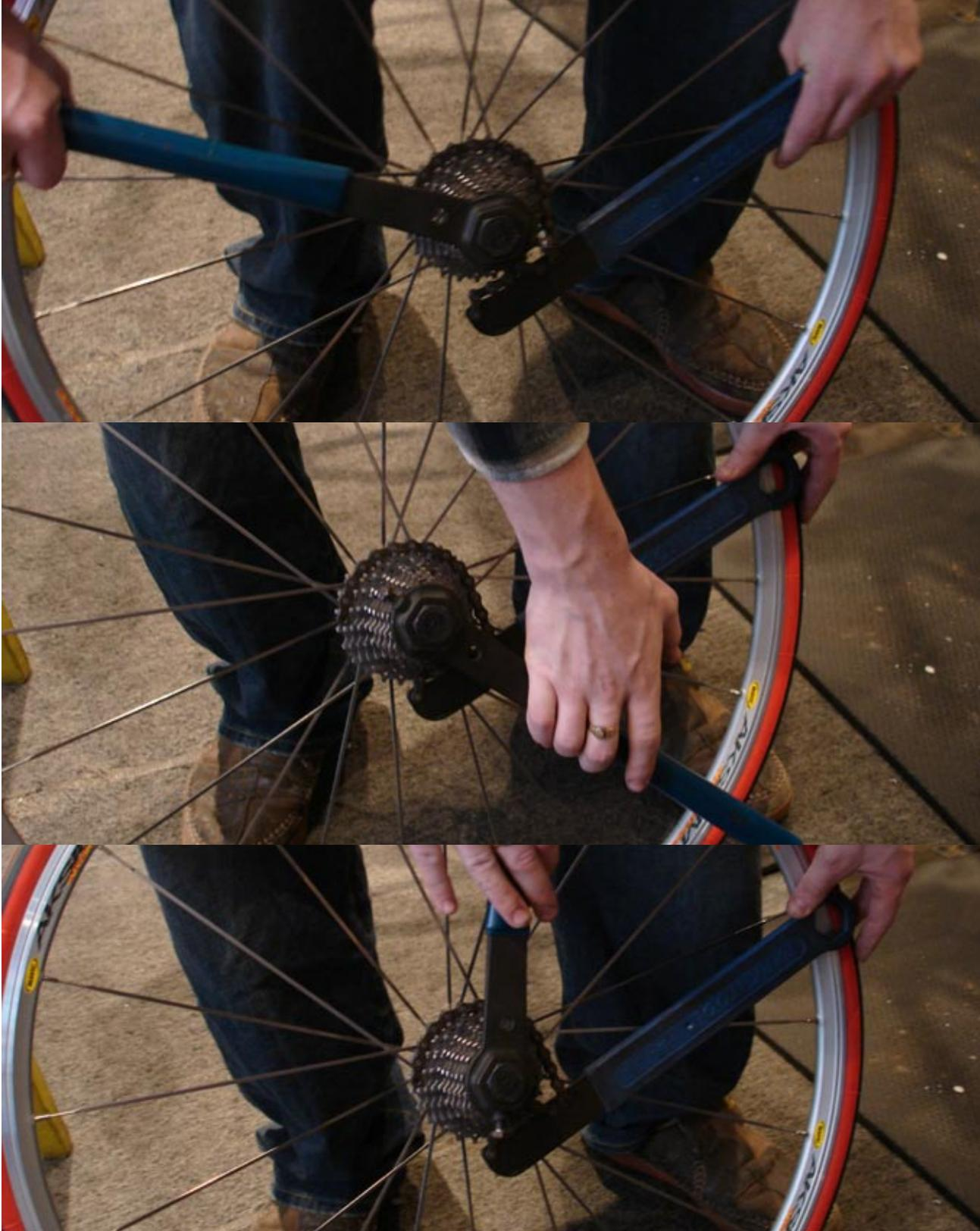
After both tools are on the cassette, hold the chain whip while pushing down on the locking tool and spinning off the lockring.
