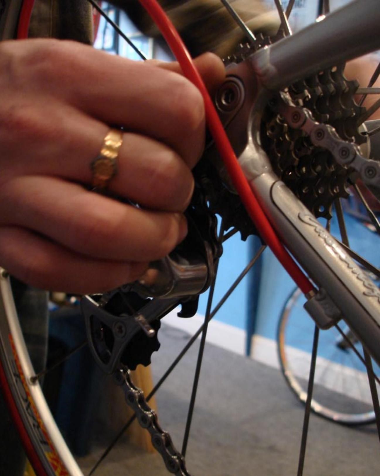
After the wheel's brake is open move to the skewer and release the handle while holding onto the wheel to have control over the wheel while taking it out of the dropouts.
