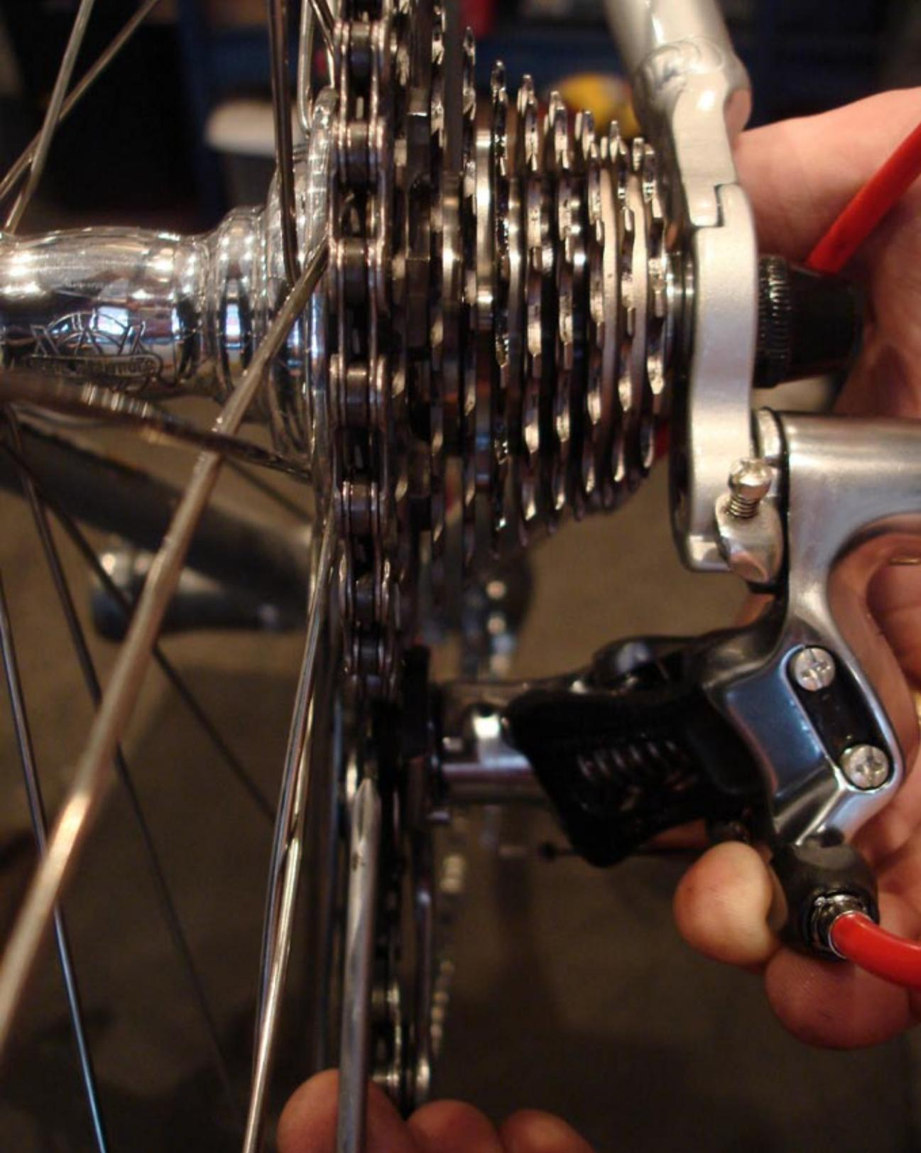
Adjust this screw in or out to have the top pulley on the derailleur line up with the last cog on the cassette.
