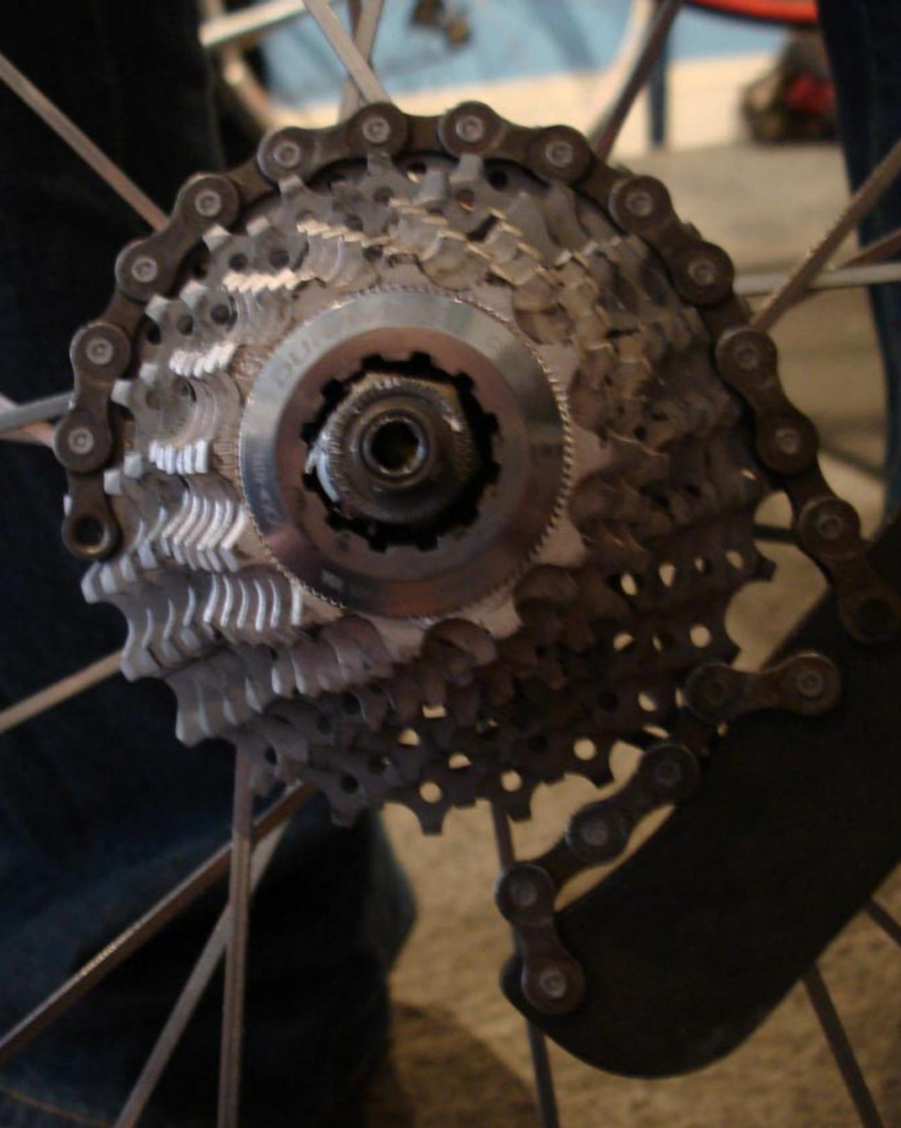
This is how your chain whip should fit on your cassette. Make sure to put as much of the chain over the second to largest cog. This is to give the chain whip as much torque on the cassette while not having the possibility of the chain running into the spokes. Also note that the tool should be in your left hand while the wheel is facing away from you.
