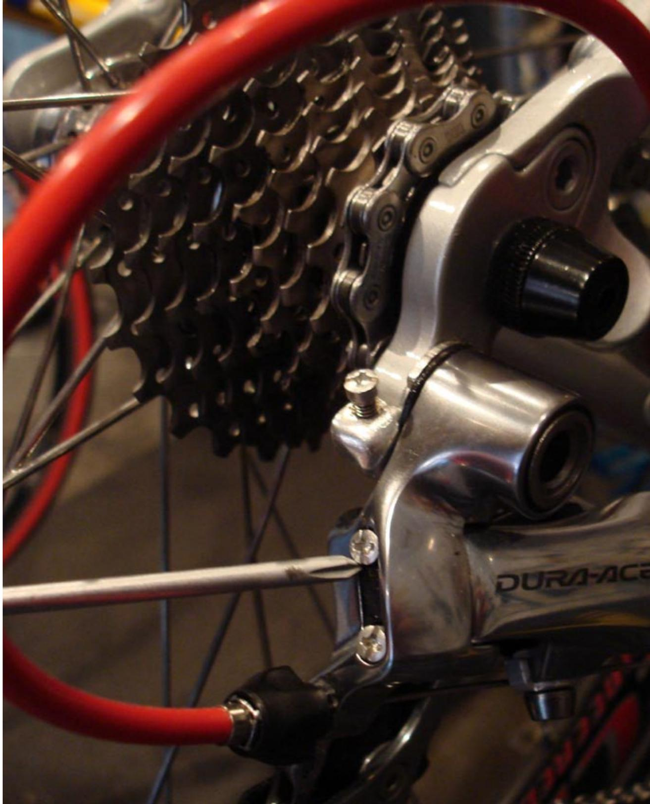
The High Limit Screw is labeled with an "H" under it or typically located as the top screw. If this is questionable look inside the derailleur itself to see which of the two screws is being touched while in the high gear.
