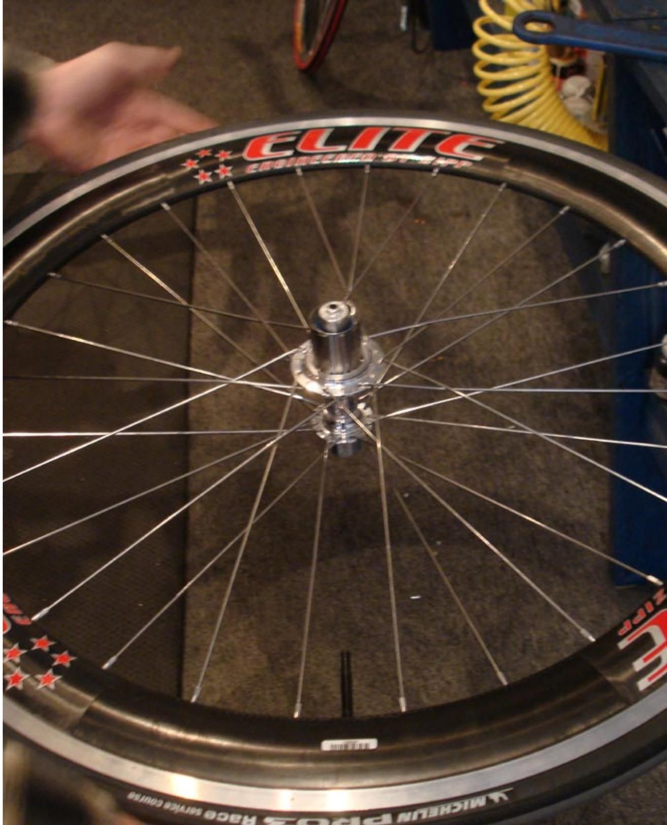
First thing to go onto the race wheel is the thin steel spacer that should be able to just fall onto the cassette body.
