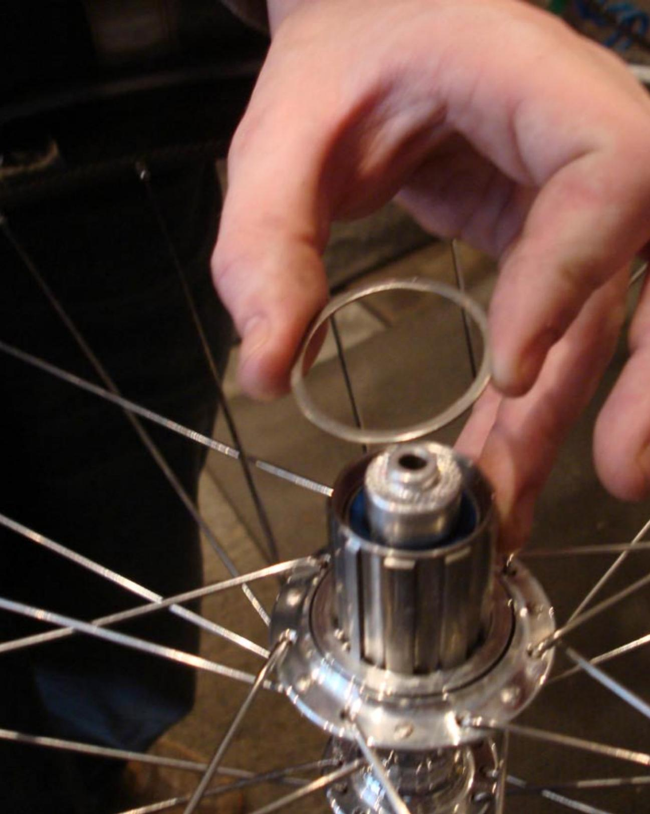
The easiest way to put a cassette on is to separate the entire cassette and put it on one piece at a time. When about to put the first part of the cassette on the body, look for the smallest gap as a guide.
